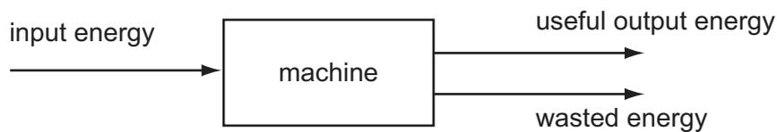
The machine is 50% efficient.
