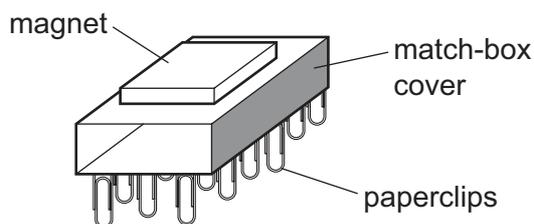
Sheets of metal are placed inside the match-box cover, between the magnet and the paperclips.
